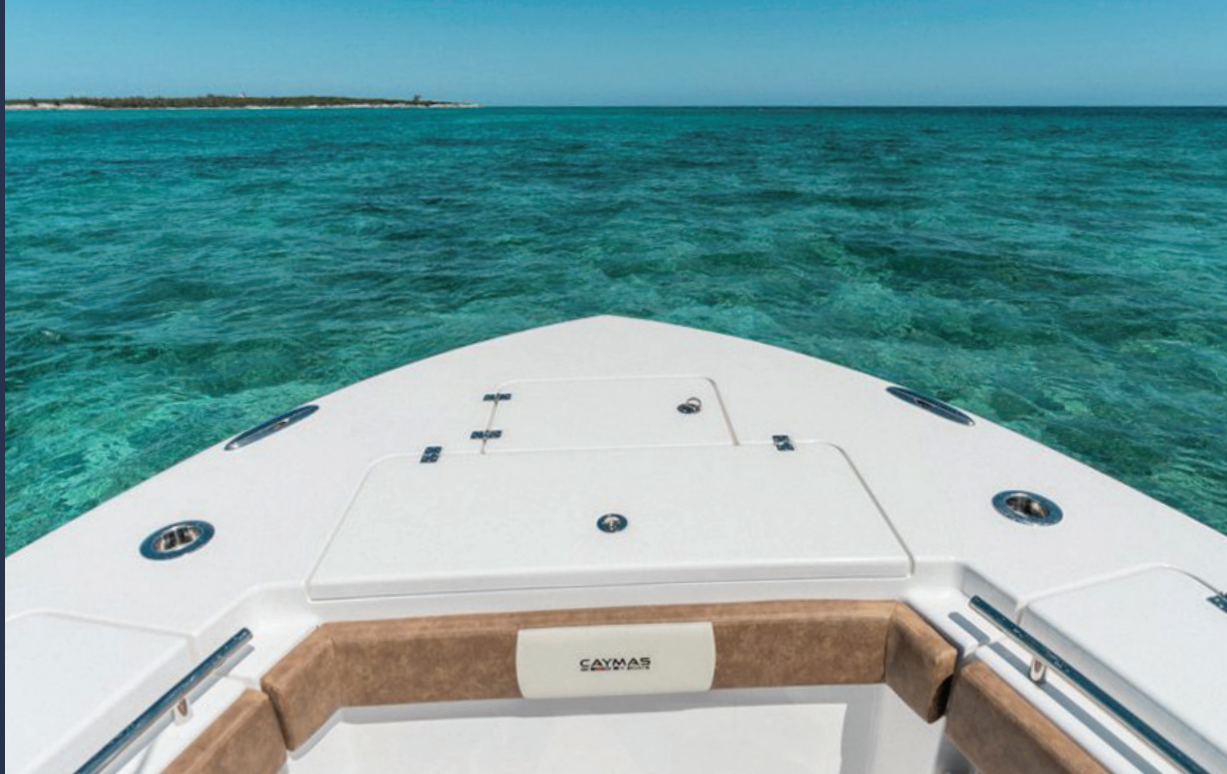
Standard anchor and windlass is concealed below the deck with controls at the helm
