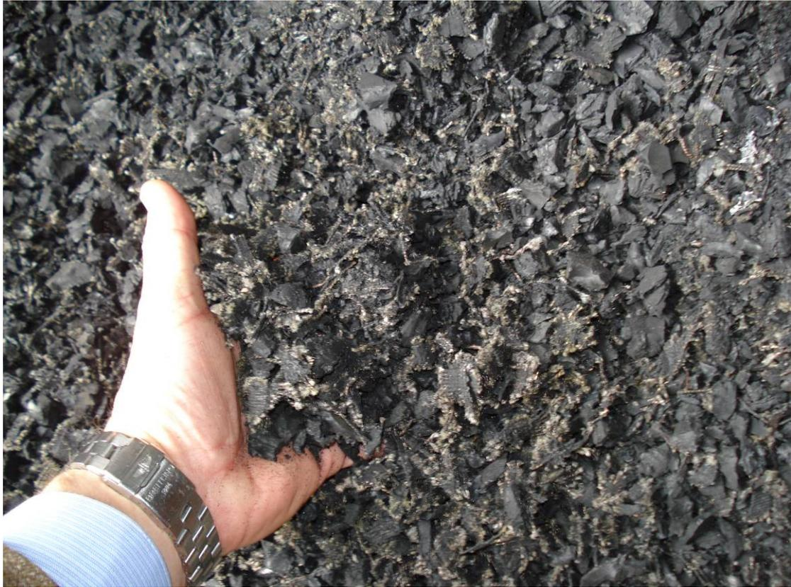
OUTPUT OF GRANULAR PRODUCT FOR THIS SYSTEM IS 4,000KG/HOUR ( 4 TON PER HOUR )
