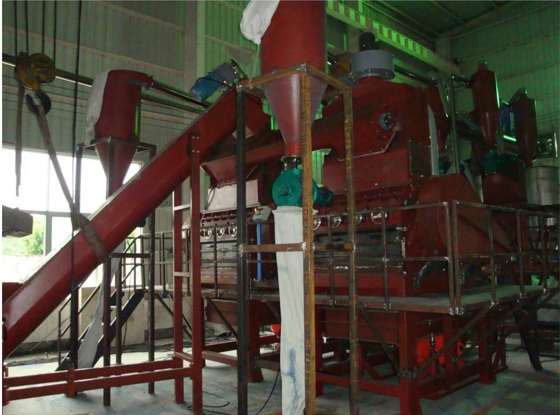
THIS IS THE SYSTEM SETUP AFTER THE AIR SYSTEM IS INSTALLED FOR FLUFF REMOVAL AND FINE DUST REMOVAL IN THE SYSTEM WHICH IS IMPORTANT TO TOTALLY ELIMINATE THE POTENTIAL OF DUST EXPLOSIONS
