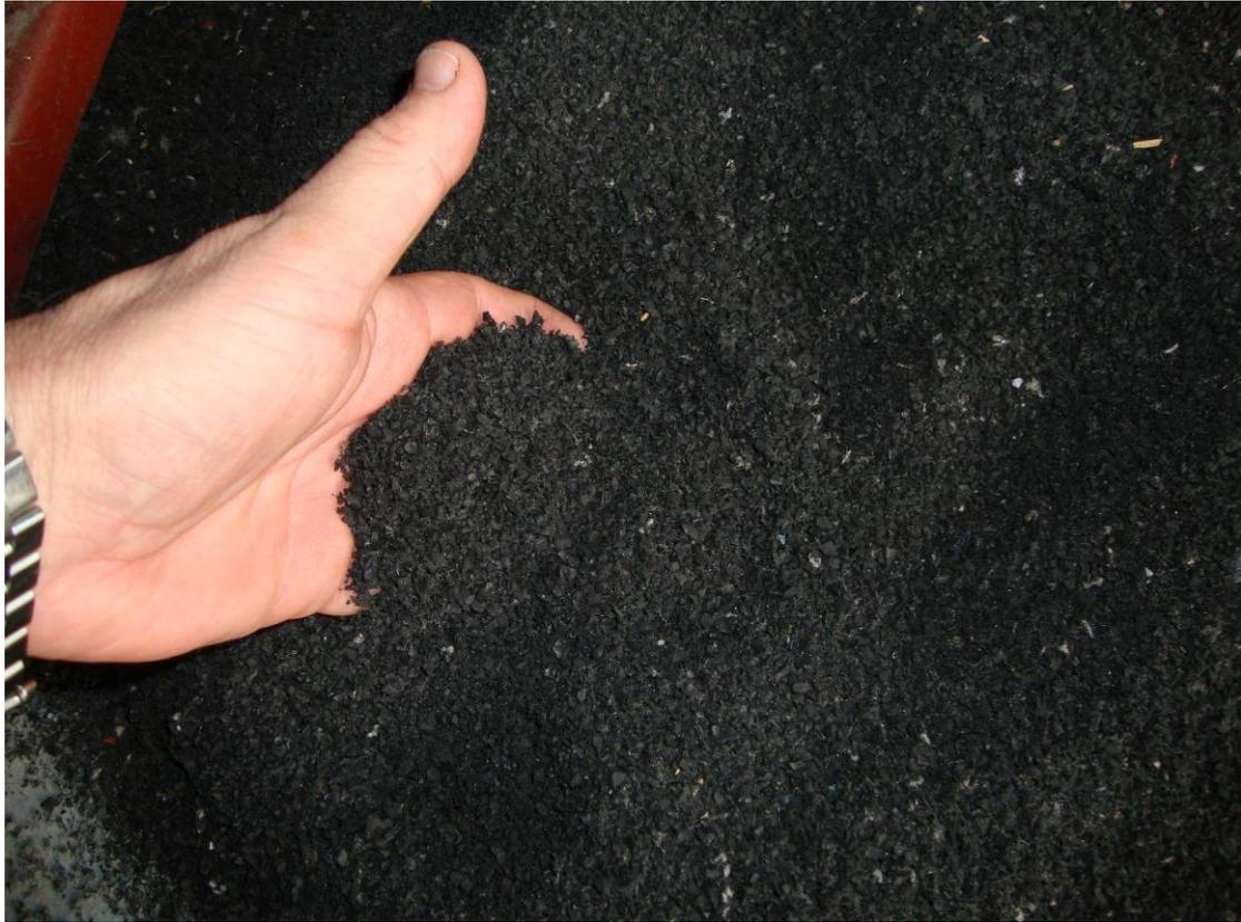
OUTPUT OF CRUM MATERIAL FOR THIS SYSTEM IS 2,000KG/HR ( 2 TON PER HOUR ) WIRE FREE AND FIBRE FREE ( LOOSE ), 8 TO 10 MESH ( 2.0 TO 2.5MM ) CRUM MATERIAL ( SCREENS CAN BE MODIFIED FOR OTHER MESH SIZES DOWN TO 15 MESH, OR FURTHER EQUIPMENT CAN BE ADDED TO MAKE FINER MESH SIZES IN THE 20 TO 30 MESH RANGE OR ULTRA FINE GRINDING SYSTEMS CAN BE ADDED TO THE SYSTEM
