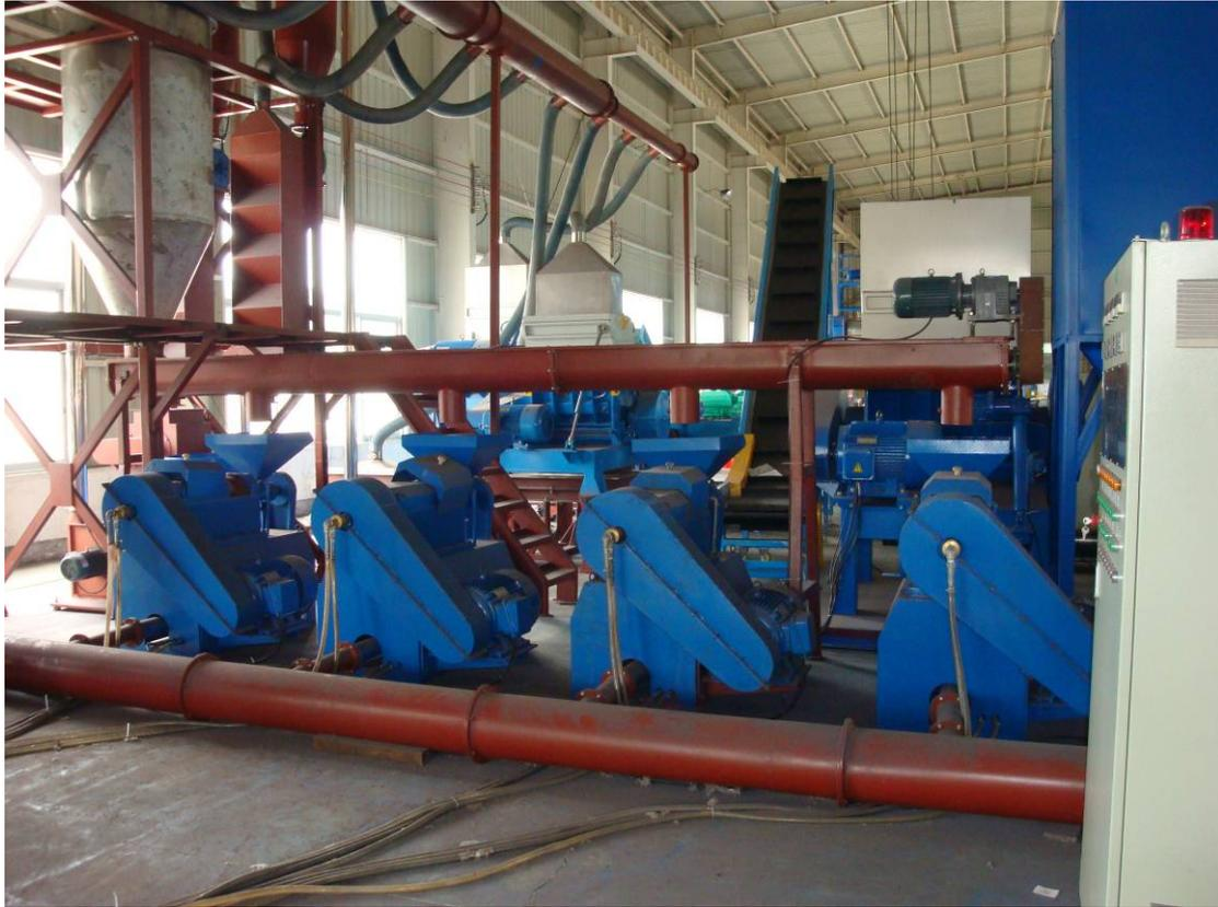
FINE GRIND SYSTEM INVOLVE MULTIPLE UNITS AND SPECIAL SCREENING EQUIPMENT TO ENSURE THAT THE PRODUCTION AND QUALITY MEETS CLIENT STANDARDS
