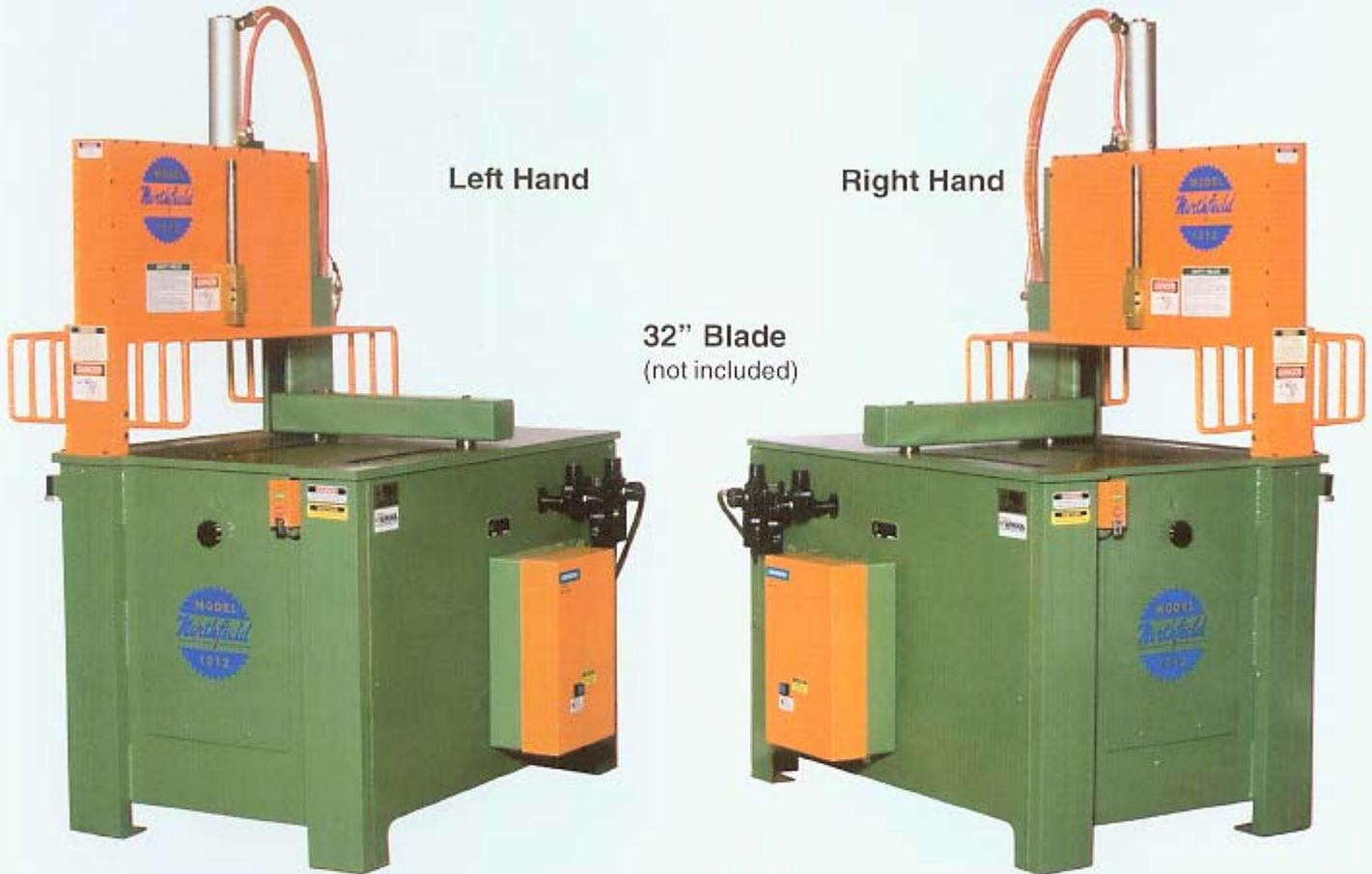
The Models 1012 & 612 are semi-automatic compressed air actuated under table cutoff saws. The blade remains in the heavy sheet steel base until the guard has the workpiece clamped. The guard remains clamped through the cut cycle until the blade is back in the base. This protects the operator from flying debris and any kickback. These saws are suitable for cutting lumber, non-ferrous metals, plastics, and various composite materials through minor changes in blade speed and feed rate.
