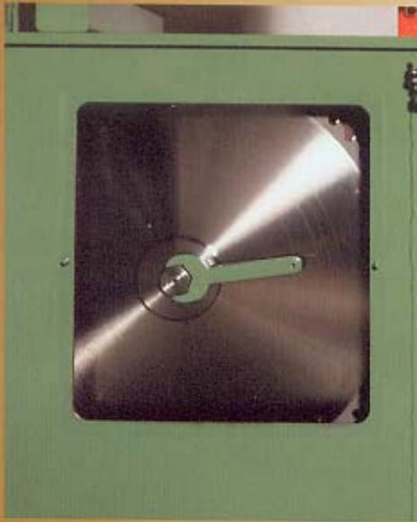
Side view showing arbor wrench for tightening the loose saw collar. A pin is provided for arbor lockup during blade changes.
