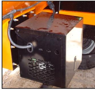
**Diesel Burner Enclosure**
