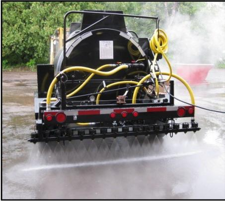
**1 Foot Sectioned Spray Nozzle Control** Allows on/off control of any 1 foot section of the spray bar. Gives outstanding flexibility in selecting spray patterns for your changing needs.
