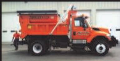
SSPH Slip In Style Asphalt Hot Boxes
