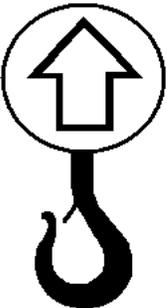
Machine may fall and cause serious damage or injury if lifted improperly. Lift only by holes in frame above.
