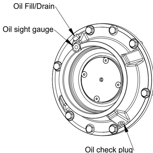
1. Rotate drum until the fill/drain plug is at bottom of drum. The fill/drain plug is the larger, square head plug on the vent side of the roller.
