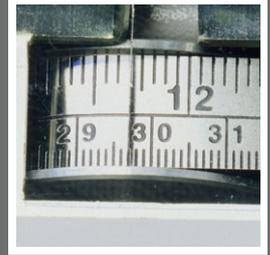
The precise measuring scale (mm/inches) for the backgauge positioning can be read easily and is located on the front table.
