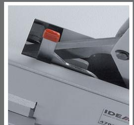
The safety catch locks the blade lever in upper position. The required two-hand operation is an important safety feature.
