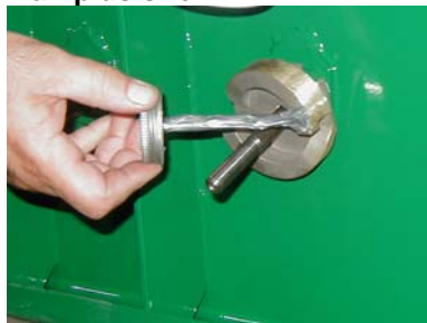
Step 5 - Apply anti-seize compound to locking ramp inclined surfaces.
