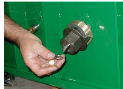
Step 9 - Install flat washer and locking nut.
