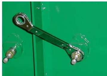
Step 10 - Using wrench (Figure 2), tighten nut until snug*.
