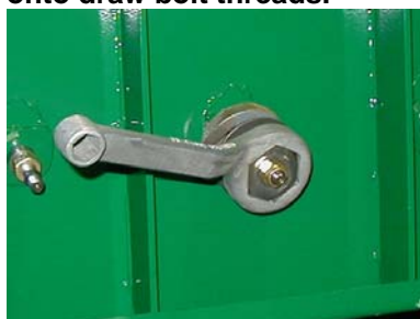
Released Position - Tensioning nut rotated fully counter-clockwise
