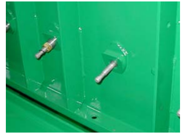
Step 3 - Push O-ring into counterbore in screen frame.
