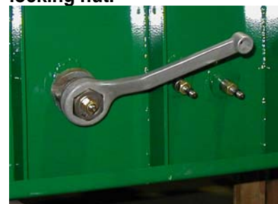
Clamped Position - Tensioning nut rotated fully clockwise.
