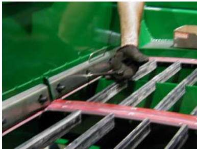
Step 1 - Insert draw bolt through frame from inside.
