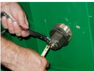
Step 10 - Pre-load spring, leaving 1/8"-1/4" (3.2-6.4mm) of draw bolt threads exposed.
