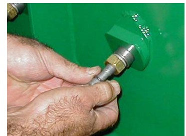
Step 9 - Install O-ring on unthreaded area of draw bolt.
