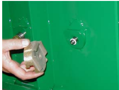
Step 2 - Install O-ring on end of draw bolt; orient locking ramp as shown
