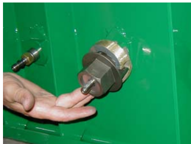
Step 8 - Slide tensioning nut onto draw bolt threads.
