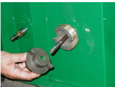
Step 7 - Orient tensioning nut.
