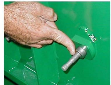
Step 6 - Push in extended washer fully to seat O-ring.
