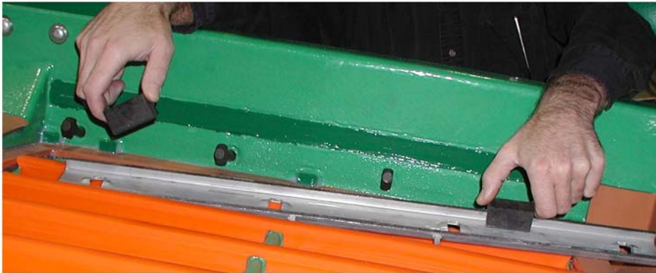
Figure 6200-2 Removing Shipping Pads From Draw Bar
