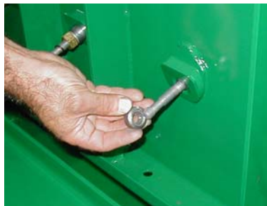
Step 5 - Orient extended washer with counterbored hole toward screen frame, and install on draw bolt
