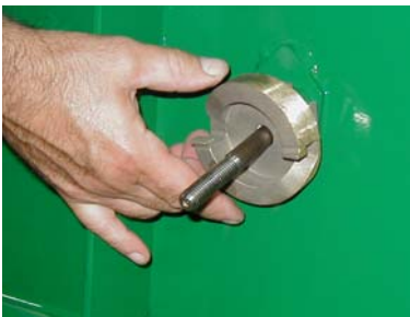
Step 4 - Push draw bolt fully through locking ramp.
