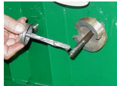
Step 6 - Apply anti-seize compound to threads of draw bolt.
