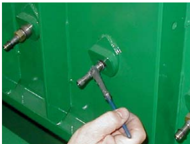
Step 4 - Apply anti-seize compound to draw bolt threads
