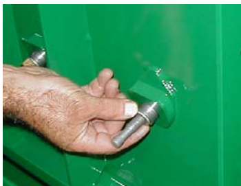
Step 7 - Install lockwasher on draw bolt.
