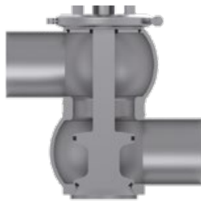
Valve type W_R (Spring-to-close, NC)
