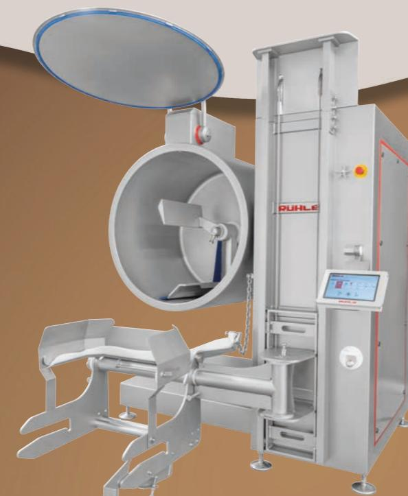
*Two independent mixing arms, a feed system and a 500 l container can process 375 l of mixing product efficiently, fast and with incredible consistency. In addition, cooling, vacuum treatment and variable arm speeds ensure optimum product yield. The secret of this success lies in its control technology, reflecting decades of experience.*
