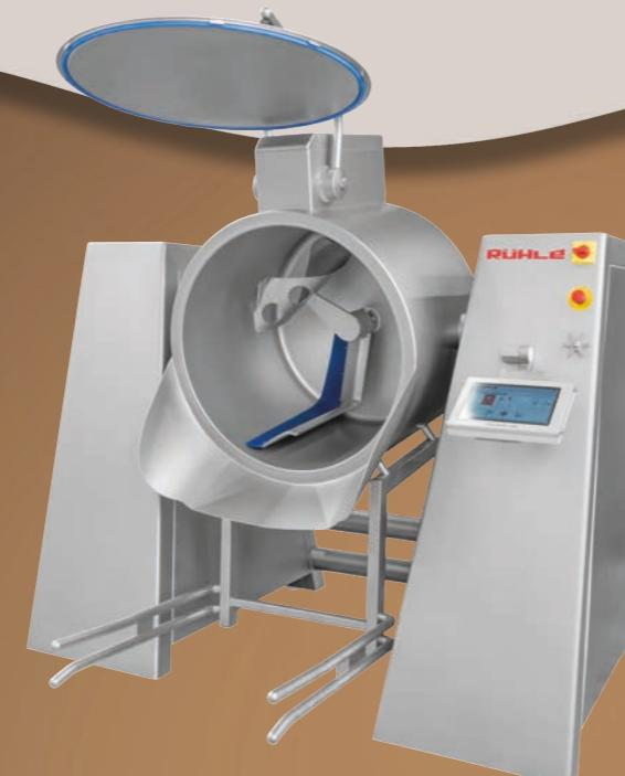
*Equipped with a fast feed system, the Original MPR 300 has a container volume of 300 l and can hold 220 l of mixing product. From cooling to vacuum treatment to variable arm speeds, this machine is perfectly designed to achieve the optimum possible results. The secret of this success lies in its control technology, reflecting decades of experience.*
