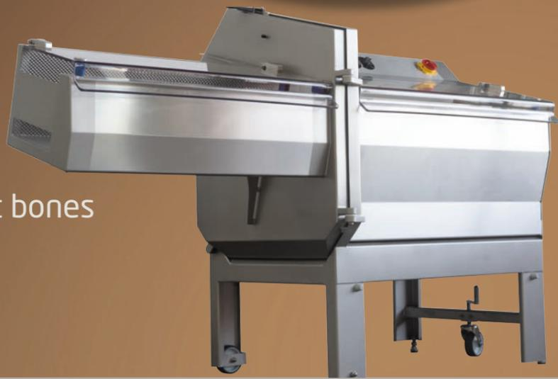
At 220 strokes per minute the Original KR 1 accurately cuts and portions chops, roulades, cordon bleu and schnitzel. Even thick - boned meat can be cut into slices of between 1 and 32 mm thickness.
