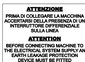
6 Information relating to the electrical connection
