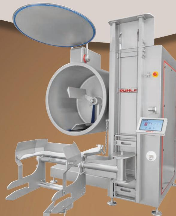
**Two independent mixing arms, a feed system and a 400 l container can process 300 l of mixing product efficiently, fast and with incredible consistency. In addition, cooling, vacuum treatment and variable arm speeds ensure optimum product yield. The secret of this success lies in its control technology, reflecting decades of experience.**
