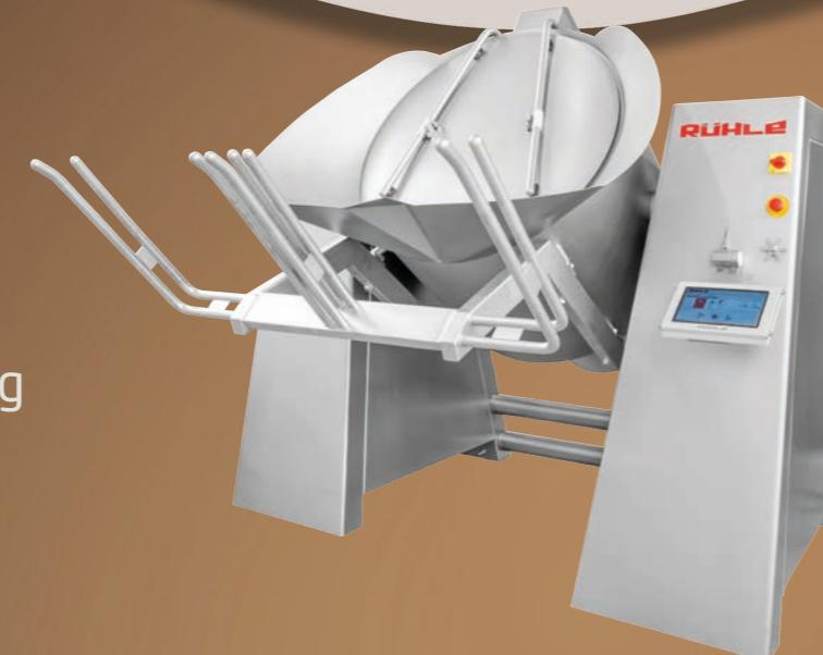
*Equipped with a fast feed system, the Original MPR 600 has a container volume of 600 l and can hold 410 l of mixing product. From cooling to vacuum treatment to variable arm speeds, this machine is perfectly designed to achieve the optimum possible results. The secret of this success lies in its control technology, reflecting decades of experience.*
