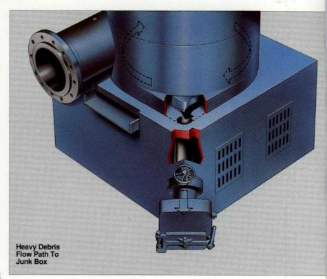
Black Clawson's new Ultra-V screen eliminates both problems with its **bottom inlet**, **patented up-flow design**.
