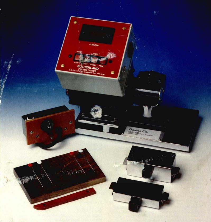
Illustrated is the Sutherland Ink Rub Tester showing two-pound and four-pound weights to which test specimens are attached, the scoring device, and an optional heated weight. The receptacle is the same voltage as the instrument. 110 volts single phase is standard. 220 volts optional at extra cost.
