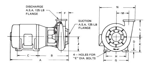
NOTES: 1. Dim. 'N' is overall width including pump and motor. 2. Dim. 'A', 'G', and 'N' may vary depending on make of motor.
