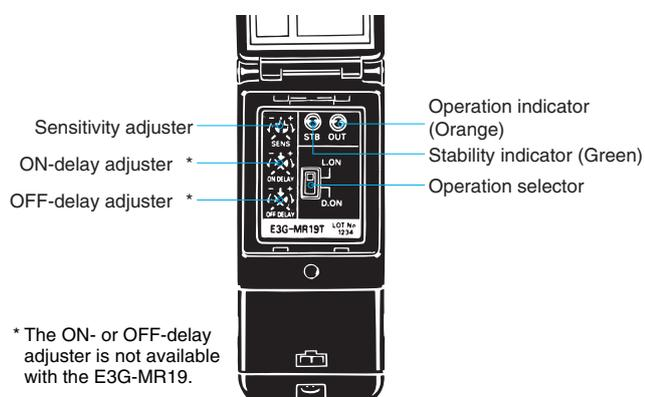
\* The ON- or OFF-delay adjuster is not available with the E3G-MR19.
