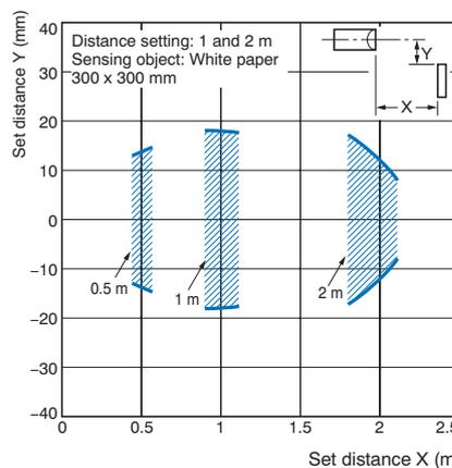
Sensing Object Size vs. Setting Distance
