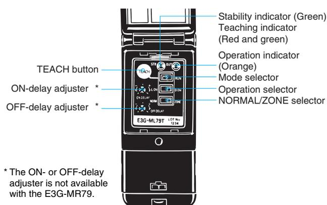
\* The ON- or OFF-delay adjuster is not available with the E3G-MR79.
