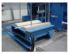
Two Coil cars for 10 ton coils
