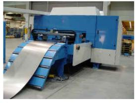
The Gripper feeder mounted on a solid steel frame as follows:
