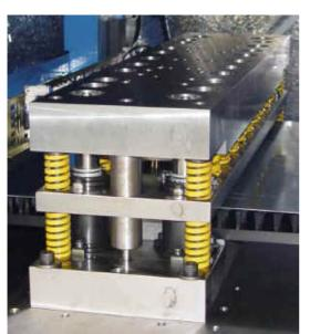
Designed for punching of large holes, hole groups, corner notching and trimming using dedicated hard tooling.
