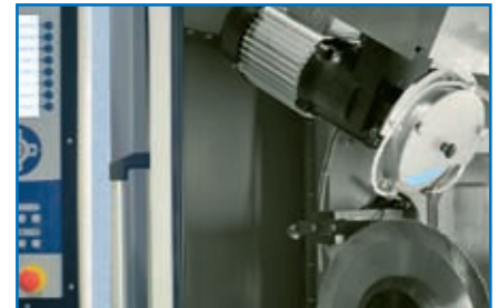
Direct drive of grinding spindle
