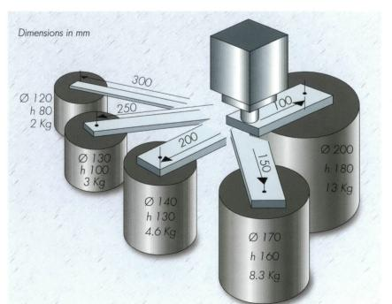
High inertia and ultra-precise positioning of the C axis.
