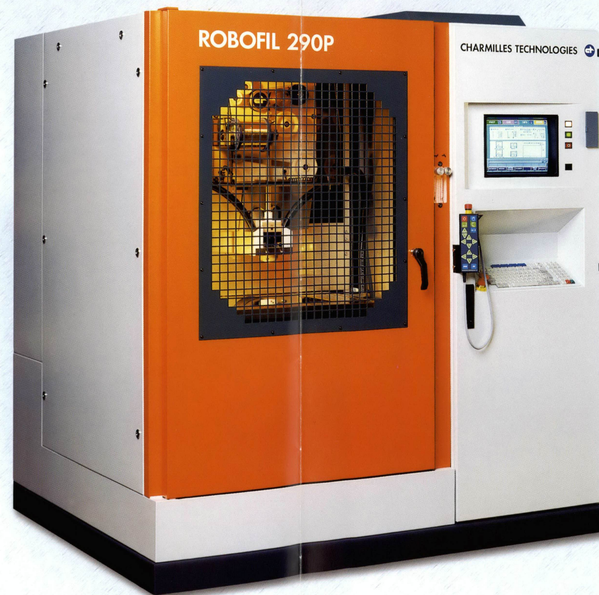
400mm X-U and 250mm Y-V travel allow for exceptional wire angles to be obtained
