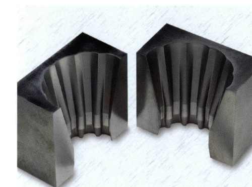
Taper-Expert maintains a constant land within 5 µm with a variable taper between 10° and 20°. This is a major factor when it comes to obtaining a perfect extrusion profile.
