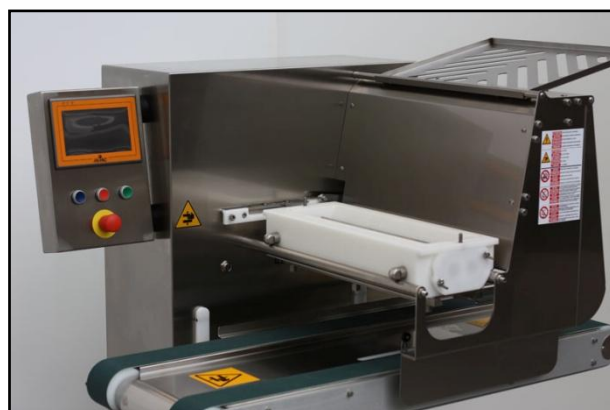
4. Carefully push the dosing group towards the structure, aligning the motor roller with the relative coupling
