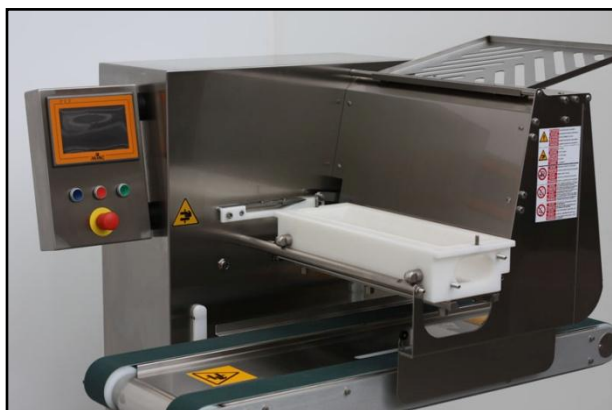
1. Lay the head on the supporting rods
