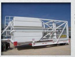
Auxiliary silo in travel position with fifth wheel, single axle, air brake system and travel lights.
