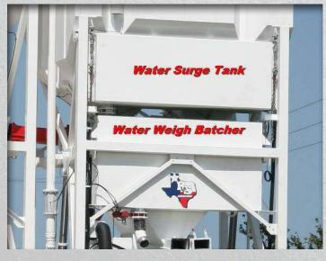
The water system includes 2" water pump with 7.5HP drive, integrated 500 gallon water surge tank with inlet / outlet butterfly valves also automatic fload switch and integrated 500 gallon water weigh batcher with outlet butterfly valve and load cells.
