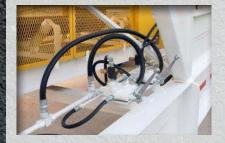
Hydraulic plant leveling system with control valves for each jack and one control valve for raising and lowering both silos.
