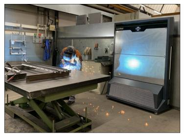
The AmbiWall is solid and cannot be opened without the use of tools. Its stable and unbreakable industrial
