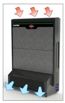
The AmbiWall pulls in polluted indoor air from overhead, filters it through two reusable KLR-bran filter elements (Keller Long Run with surface membrane), and releases cleaned air at the bottom. As an additional option, a HEPA filter H13 or H14 according to EN 1822 for capturing ultra-fine pollutants can be installed inside the air outlet.
