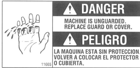
Figure 4 — Danger label, removed guard
