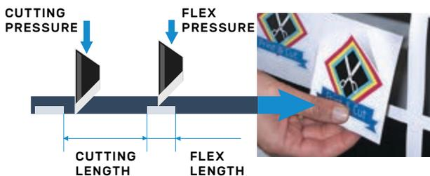
Alternately, one length is cut completely through the material, and one length is cut halfway through. This way a kind of tear-off line is created, ensuring the material keeps a certain rigidity during transportation through the Summa cutter, while remaining easy to remove from the design afterwards.
