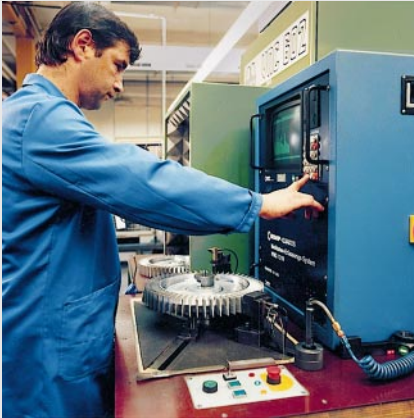
Electronic check of the dimension accuracy of an ELMO-G impeller.
