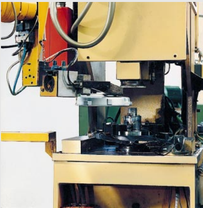
Fully automatical final check of endshields of ELMO-F and -G drives.
