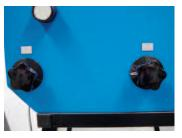
Nip and pull roller pressures are adjusted independently for best results.
