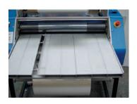
A fully adjustable, positive side lay is provided to aid consistent feeding by hand. The feed table can be easily removed to allow the coupling of an automatic sheet feeder.
