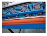
A twin bank of cooling fans is supplied to enhance film clarity and aid clean side trimming.
