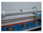
Films with either 57mm or 75mm cores may be used for flexibility of supply.
