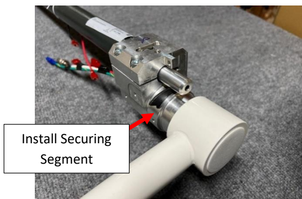
Figure 20: LCH Light Head with Camera - Install Securing Segment
