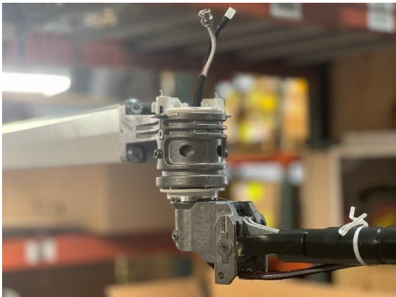
Figure 17: Mounting the LCH Spring Arm with Camera
