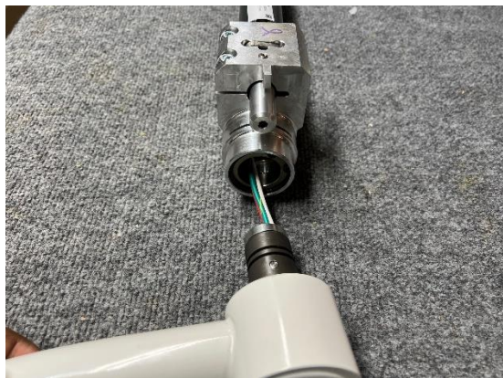
Figure 19: LCH Light Head with Camera Install
