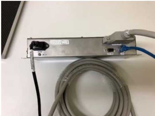
Figure 7: View of the DR power box connection and the tethered DR Panel
