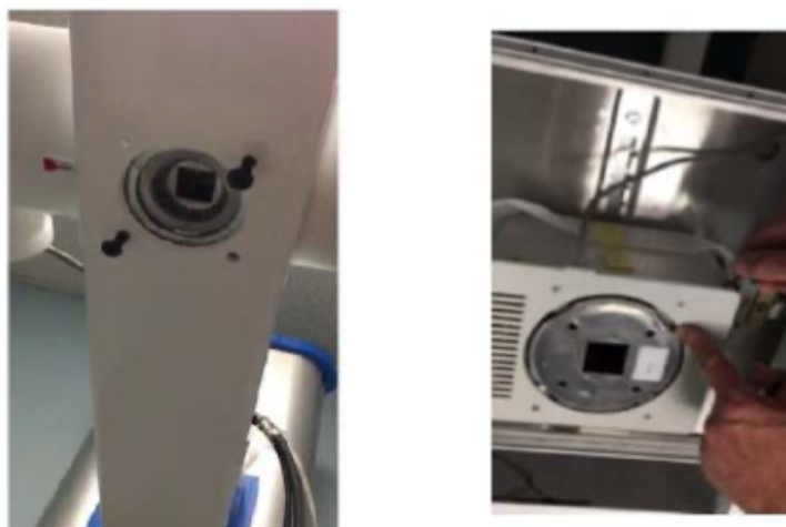
Figure 3: showing the 4 mounting holes at the bottom of the arm to mount the tube and ring
