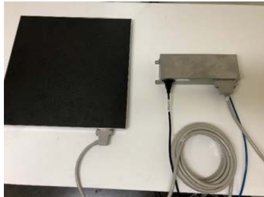
Figure 7: View of the DR power box connection and the tethered DR Panel
