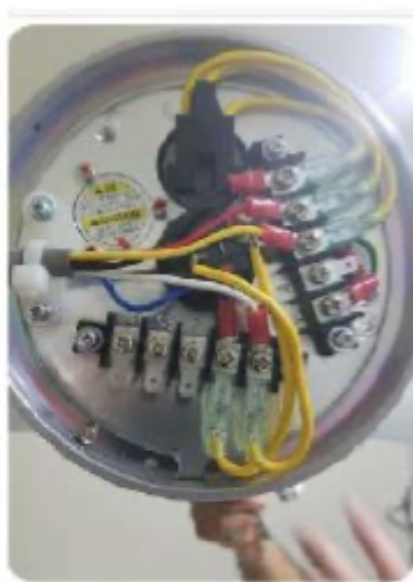
Hooking up Wiring to Tube Black is 1, Red is 2, Yellow is 3, White is 5 and Blue is 6
