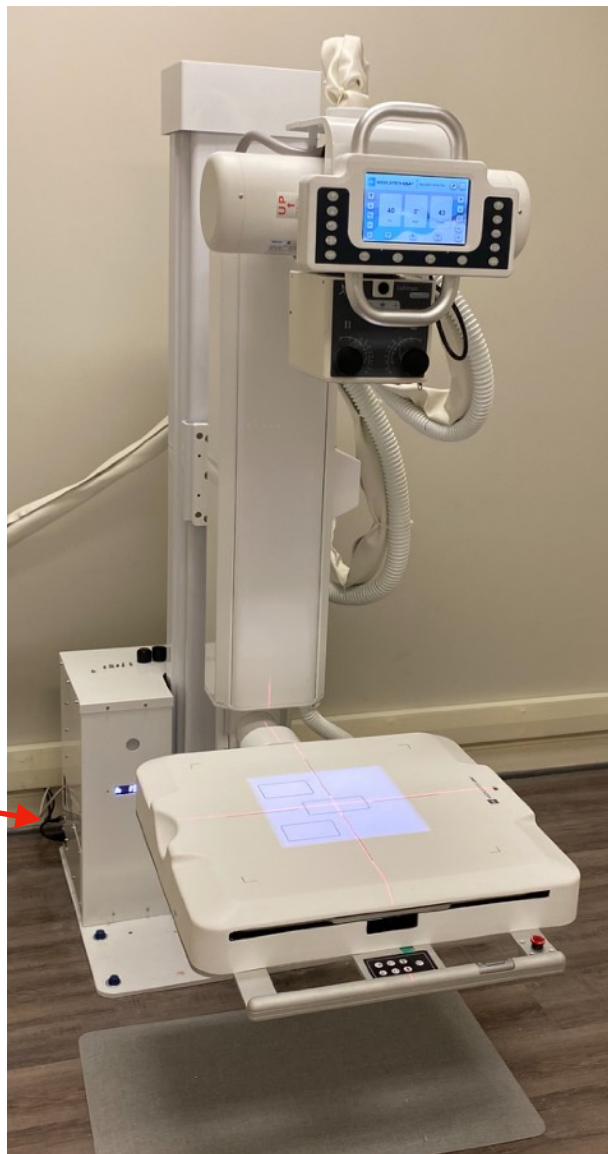
Figure 8: MX40 showing manual power switch location
