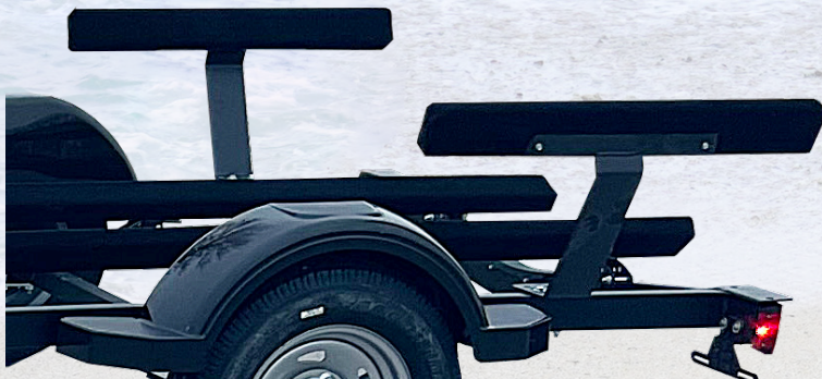
Bolt to Frame Side Guide Ons 11" Tall Bracket, 32" Bunk, Part # 1805-SG11
