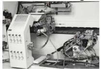
It carries out the **rounding** of straight and shaped edge angles and the **trimming** of the upper/lower panel side
