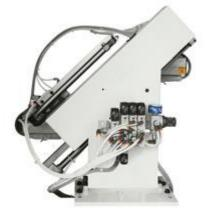
It carries out the cutting of the front and rear exceeding edge (also for post/soft formed panels).
