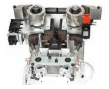
It trims the panel edge obtaining a perfect uniform surface for the glue application and a perfect jointing line with the edge.
