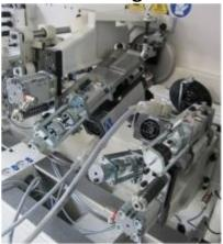
It carries out the trimming of the top and bottom exceeding edge
