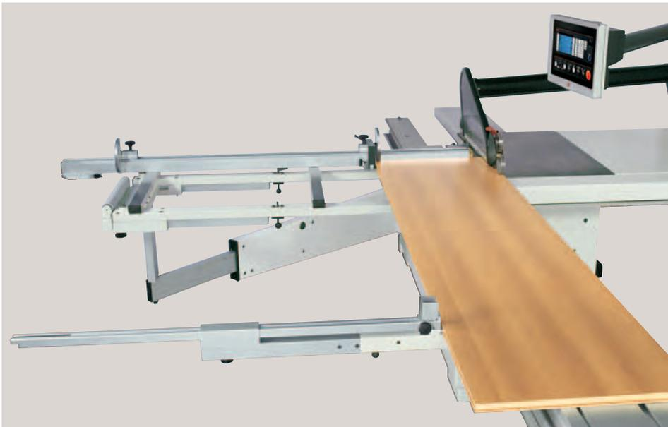
Rip fence unit with exclusive referencing system for the first trim cut which allows to set the trim quantity to be cut for every side.
