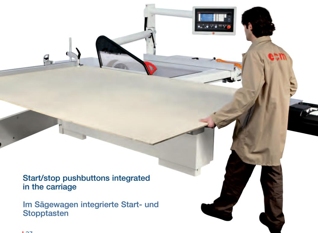
**Start/stop pushbuttons integrated in the carriage**
