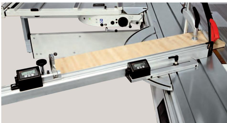
Fence for angled cutting with **mechanical self-adjustment** of the cutting size in relation to the blade. Detecting system on magnetic band and readout on LCD graphic display both for frame and angles and stops positions on squaring fence.
