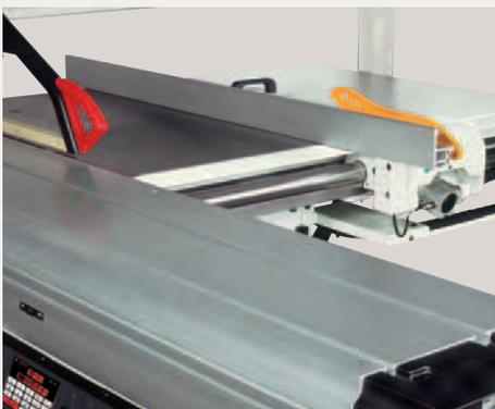
**Parallel fence with electronic positioning**
