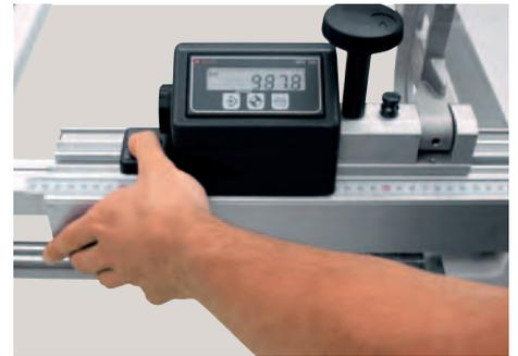
The two mobile stops and the fixed stop are equipped with readouts on LCD display and position detecting system on magnetic band: **precision and easy to use.**
