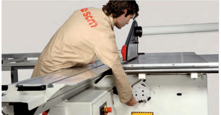
**Vertical and horizontal adjusting system of the scoring blade** with mechanical stops for a rapid repositioning. The lever mechanism position allows to carry out the adjustment directly from the machine front.
