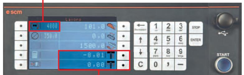
**Automatic (vertical and horizontal) scoring unit adjustment** with a +/- 0,01 mm precision
