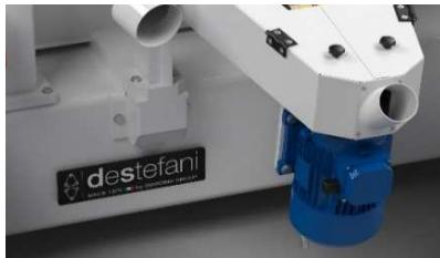
Sanding unit for flat edges or profiles, with air cushion pad, counter shaped in respect to the profile to be sanded, with pressure that can be regulated.
