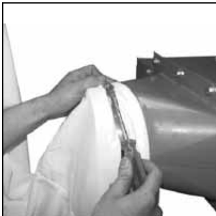
25. Place inlet of filter bag to 8" outlet and tighten it with 8" bag band.
