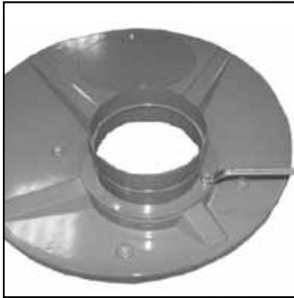
19. Fasten hose connector to cover with four 5/16 X 1" screw, four 5/16" flat washer, four 5/16:" lock washer and four 5/16" hex nut.
