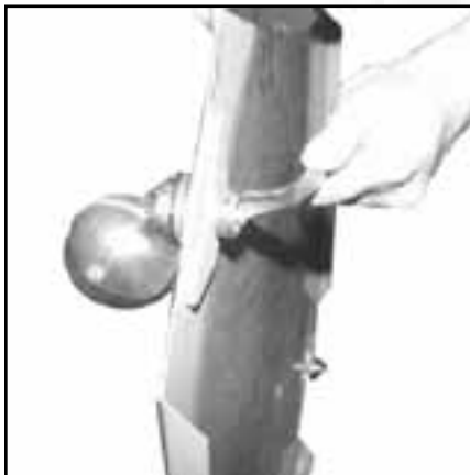
26. Assemble the wheel to collecting drum base with 3/8" hex nut and 3/8" flat washer.
