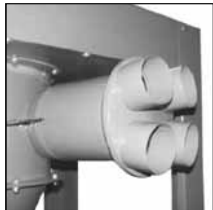
17. Position the 4 inch x 4 holes inlet housing to 8 inch inlet of blower housing. Align holes in inlet housing with pre-drilled holes in inlet and fasten with three pan head screws.
