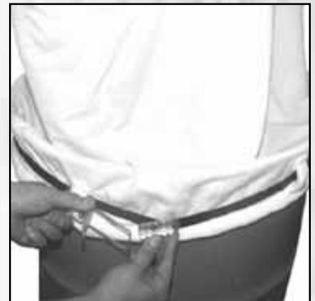
28. Position bag filter on 50 gallon drum and tighten it with bag band as shown.
