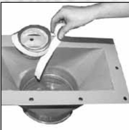
15. Remove the paper backing and start the gasket material around the outer edge of outlet and continue until a complete turn.
