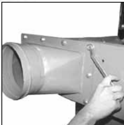
16. Position outlet to the blower housing, and align holes. Fasten with ten 3/8" x 1 inch-long screws and ten 3/8" flat washer.
