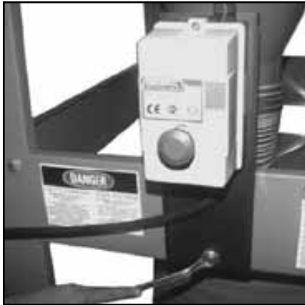
22. Assemble switch panel on the support bracket with two 3/8" x 3/4" screws, four 3/8" flat washer and two 3/8" hex nut.
