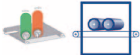
UniSander 2.2.0. 0-15° Surface sanding – light profile sanding. In / Outside.
