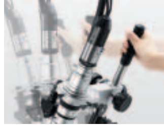
Observation from various angles by moving the pole.
