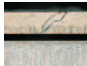
Horizontal two-part split Razor (2000x)
