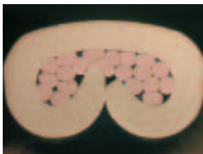
Connector crimp (100x)
