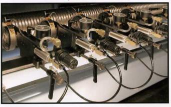
EMT knives are pneumatically activated and can be easily adjusted in 1/2 inch increments along the web to provide a superior cut. Alternative knives and cut width increments are available.
