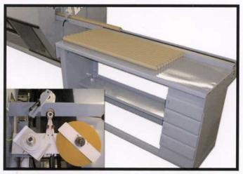
Cores are loaded on the optional offset staging table and automatically indexed to the core infeed conveyor. A larger capacity core hopper is also available as an option. Photo inset shows an optional tape to core system that secures the tails to the cores with an adhesive.
