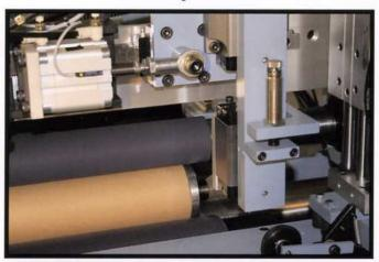
Jennerjahn's shaftless rewind system eliminates the need for any rewind mandrels. Chucks are activated to secure the cores during the winding process. Chuck tips for 2 - 4 inch O.D. cores can be easily interchanged.
