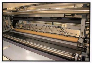
The autoloader transfers the cores to the winding station utilizing a pick and place vacuum device. The machine will continue to operate in a fully automatic mode as long as cores are in the hopper and the unwind stand is loaded with product.
