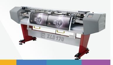
The Fotoba Dreamcut XLD-170 offers an automatic finishing solution for trimming and X/Y cutting. Equipped with digital sensors, it compensates feed misalignment for a perfect cut. The Fotoba Dreamcut XLD-170 is ideal for cutting large quantities of posters, photographs, canvas, vinyl, and laminated materials up to 40 mil thick.
