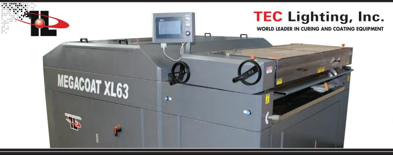
The MegaCoat XL is the large format UV coater for todays wide format printer. The MegaCoat has the ability to apply a wide range of UV coatings specifically designed top address the challenges that wide format printers face when it comes to enhancement and protection. UV coating can increase color vibrancy, reduce the appearance of "Banding" and help protect against the elements including chemical and UV light.
