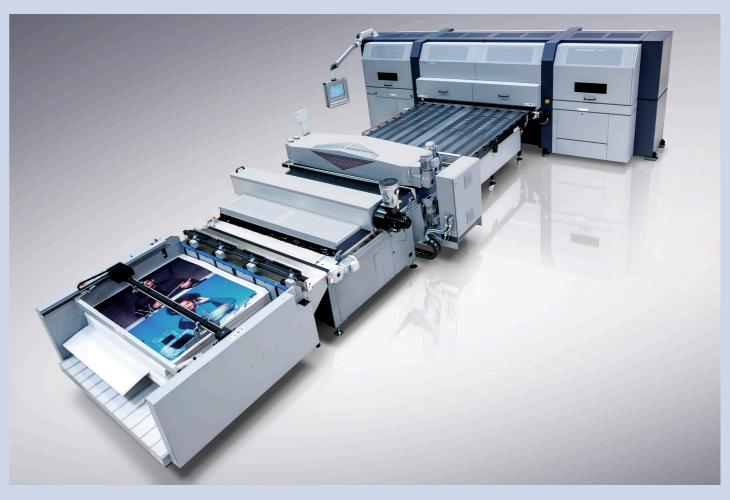
The Rho 1000 is ideally suited for integration into existing production systems and is capable of achieving a production output of up to 500 m² per hour, without interruption, around the clock, whilst ensuring optimum quality. The continuous production system has, at its core, the highest precision media transport mechanism available which, unlike table systems, features a unique continuous vacuum belt.
