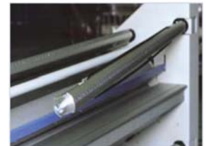
Cantilevered Supply Shaft*
