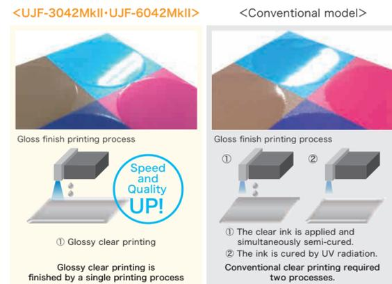
Mimaki clear control (MCC) has been newly added to the UJF-3042/6042MkII models. In order to minimize dust adhesion and air bubbles on the print, MCC shortens the ink curing time by processing the clear ink print and UV-light irradiation simultaneously. MCC provides a gorgeous gloss finish.
