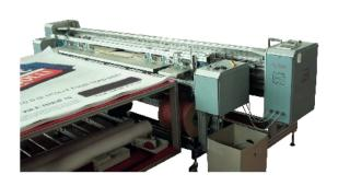
The zipper accessory enables a fully automatic workflow for cutting and applying the zip to digitally printed wide format posters. Just after the cut is done the zip is applied perfectly parallel to the image.
