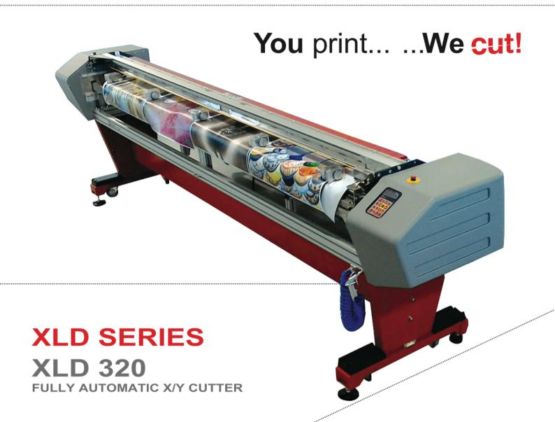
Superwide X/Y cutter made for non-stop production with modular accessories system
