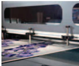
An automatic alignment bar helps you quickly position media, the printer measures its thickness, and an onboard camera detects the position of loaded media.<sup>5</sup> Print up to 4 sheets at once.
