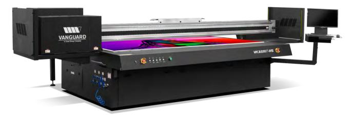
The VK3220T-HS redefines the meaning of productivity on a  $3.2 \times 2$  meter ( $126" \times 80"$ ) UV-LED flatbed. With up to three rows of printheads, print speeds can reach over 3,800 square feet per hour. Utilizing 4 picoliter drop size Kyocera heads and a high-speed magnetic drive, there's no compromise on speed to achieve remarkable quality. With the ability to print up to 10cm thick, the only limitation is your imagination.
