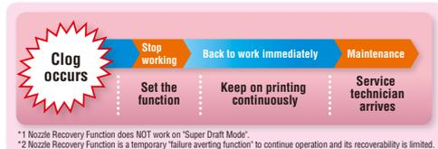
\*1 Nozzle Recovery Function does NOT work on "Super Draft Mode".
